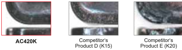
Work Material: GGG-40.3, Toolholder: PCLNR2525-43 Insert: CNMG120408 Cutting Conditions: v_c = 350 m/min, f = 0,25 mm/rev, a_p = 1,5 mm, wet
